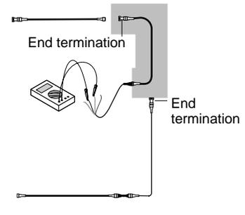
4. **Check the condition of the sensing cable.** Measure the resistance between the black and green wires of the leader cable.
