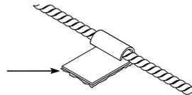
4. **Test** each length of sensing cable after installing it and before attaching it to cable already installed. Confirm that the sensing cable is clean and intact by following the Sensing Cable Test Procedure detailed on page 6.
