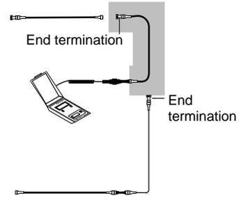
4. **Check the condition of the sensing cable(s),** again following the PTB operating instructions. If the sensing cables are clean and free of contamination, the current measured should be below 10  $\mu\text{A}$ . *If the reading exceeds 10  $\mu\text{A}$ ,* use the PTB to locate the liquid or contamination and take appropriate corrective action.
