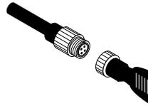
2. **Orient** sensing cable so end termination will be away from connection to the TraceTek alarm module. Work out from the alarm module connection. For sensing cable on reels (lengths over 10 feet), put the reel on an axle and pull the cable out.
