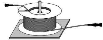
3. **Install** sensing cable in accordance with the engineer's leak detection layout plan.
