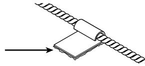
4. **Test** each length of sensing cable after installing it and before attaching it to cable already installed. Confirm that the sensing cable is clean and intact by following the "Sensing Cable Test Procedure" on page 5.
